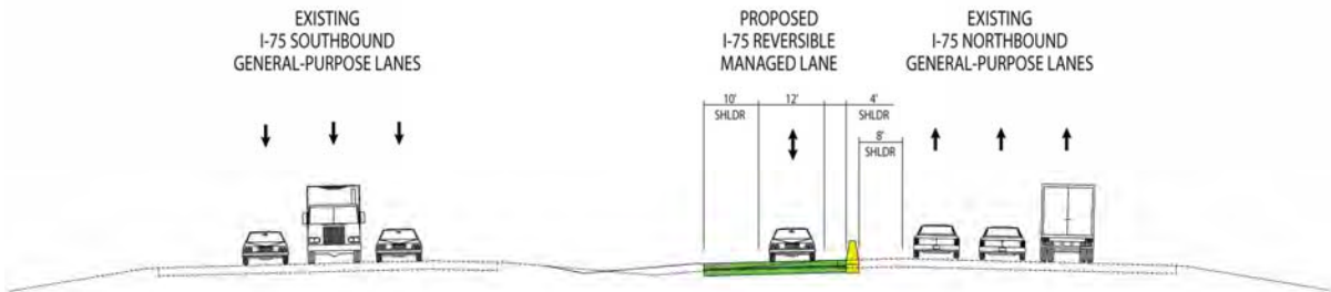
Figure S-6. I-75 Managed Lane (North of I-575) – Looking North
